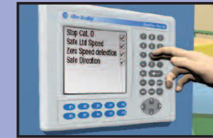
Safe-Speed Control functions configured at setup using standardised approach independent of platform chosen.
