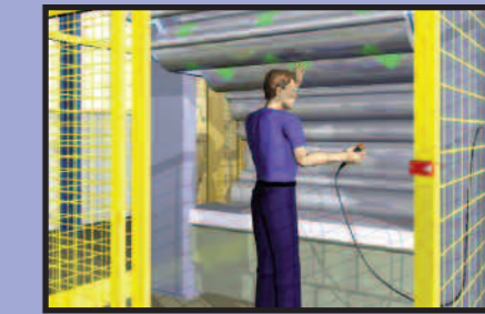
Operator uses a 3 position enabling (grip) switch to control the safe limited speed of the motion while carrying out cleaning/maintenance. Gripping or releasing the enabling (grip) switch will initiate a safe stop.
