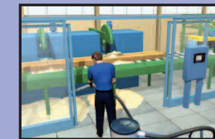
Once zero speed is detected (saw blade is at standstill), and the machine is in stop mode, the guard door is automatically unlocked to allow operator access.
