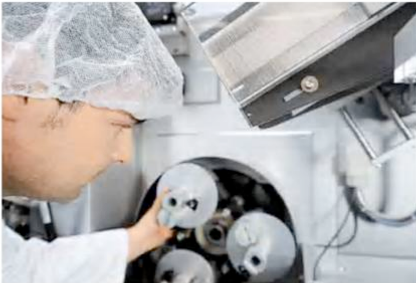
Inspection of the carton pick-up by one of Uhlmann's support service technicians - regular, scheduled maintenance is an investment in machine reliability.
