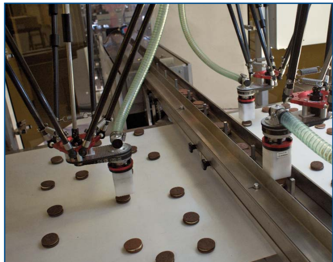
Vision-guided robots is quite common. In this cookie sorting application, the robots place different shaped cookies into a blister tray for packaging. The imaging software (top left), based on the Matrox Imaging Library, will help determine the correct shape of the cookie, index it so as not to overfill the tray, and (above) send coordinate information to the robot. Images courtesy of Bosch Packaging Technology.
